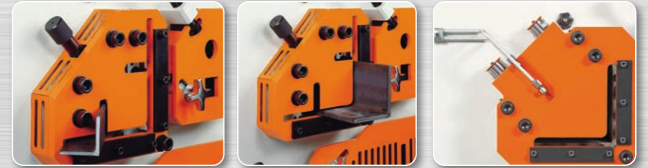
*Optional hydraulic hold-down for angle shear.
