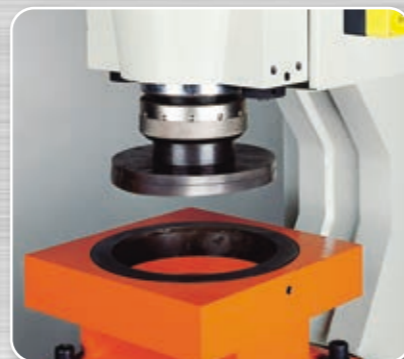
*Oversize punch attachment. Safety cover removed for showing.
