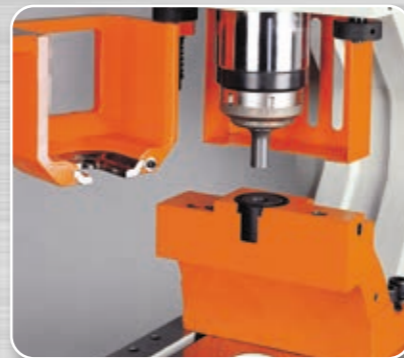
*Goose-neck die holder for punching channel flanges and webs.
